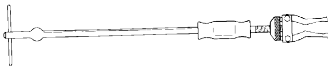
Puller Bolt 91-85716 and Puller Jaws 91-46086A1
