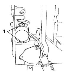
Rotate TPS fully clockwise (holding throttle shaft in closed position). On models with ECM P/N 14623A15 and above, voltmeter should read .200 - .300. If readout is not within specifications, adjust TPS to obtain readout of .240 - .260.
