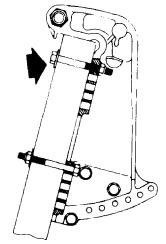
Install upper bolts so that hex head end of bolts is on the inside of boat transom.
