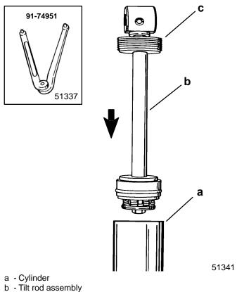
c - End cap (Tighten securely.) Use spanner wrench.
