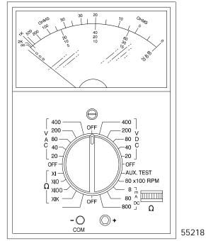
**NOTE:** Volt/Ohm Multi-Meter 91-62562 can be used to test ignition system voltages if used in conjunction with DVA ADAPTOR 91-89045.
