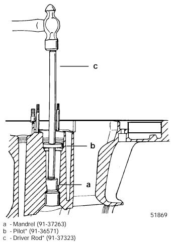
\*From Bearing Removal and Installation Kit (91-31229A5)
