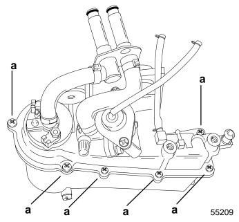
a - Screws (4 screws are hidden on back side)
