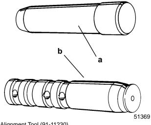
a - Alignment Tool (91-11230) b - Shaft 2. Align tilt ram and housing using alignment tool.
