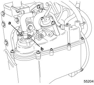
a - RED (+) Terminal [Torque nut to 6 lb. in. (0.7 N·m)] b - BLACK/RED (–) Terminal [Torque nut to 8 lb. in. (0.9 N·m)]
