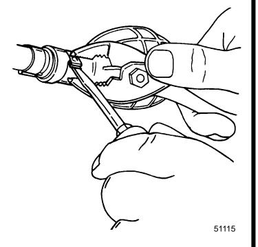
2. To install fuel line clamps, grip hose clamp with pliers and push down on hook with screwdriver until hooks interlock.
