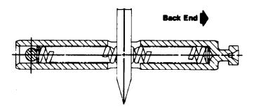
Clutch Actuator Rod with One Additional Shim Washer Added to Back End
