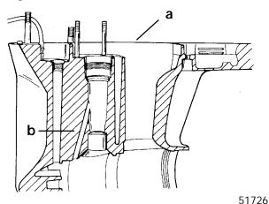
a - Late Model Gearcase Without Lubrication Sleeve
