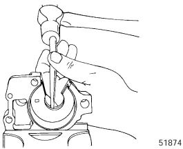
b. Drill two 3/16<sup>2</sup> (4.8mm) diameter holes thru the top of water pump cover (but not thru insert). Drive insert out of cover with a punch and hammer.
