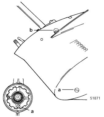
a - "Fill" Screw (Sport Master Gear Case has Drain/Fill Screw Located in the Bearing Carrier)
