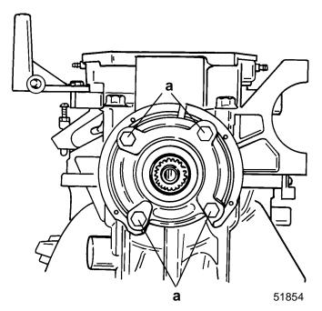
a - Crankcase Attaching End Cap Bolts
