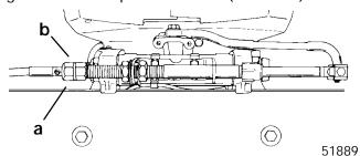
a - Cable Attaching Nut b - "V" Groove
