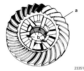
a - Reverse Gear Teeth b - Clutch Jaws
