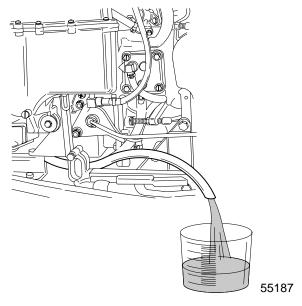
**Results:** Fuel flows freely from pulse pump inlet hose. Remove, disassemble, and inspect pulse fuel pump (section 3).
