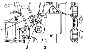
3. Reconnect WHITE/BLUE lead to detonation sensor (200 model).
