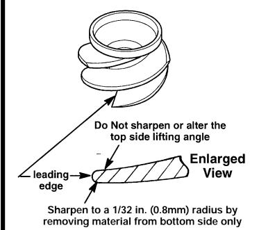
The intake of gravel through the pump can round off and wear the leading edges on the impeller. Some conditions you may experience from a worn impeller are (1) a noticeable performance loss, especially on acceleration, (2) difficulty getting the boat on plane, or (3) an increase in engine RPM at wide open throttle. Check the impeller blades occasionally for damage. Use a flat file to resharpen the leading edges as shown.
