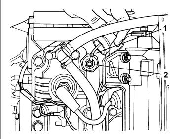
2. Outboard running in gear, advance throttle arm until maximum spark adjustment screw (1) contacts spark stop (2), at about 2500 RPM. Adjust maximum spark adjustment screw (see specifications) if necessary. Tighten locknut (3) and turn engine off.
