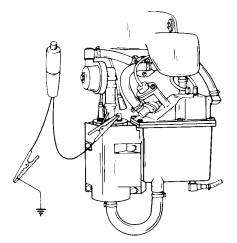
STEP 3: Perform fuel injector test procedures (outlined) while depressing remote starter switch.
