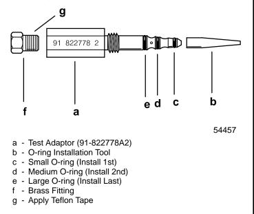
4. Install test adaptor 91-822778A2 into manual release valve hole.
