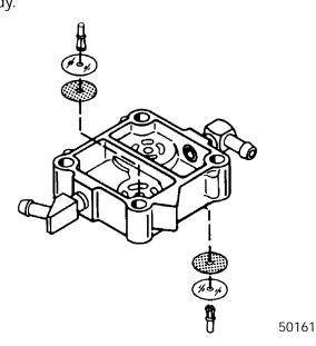
3. With retainer installed in pump body, break retainer rod from retainer by bending sideways.
