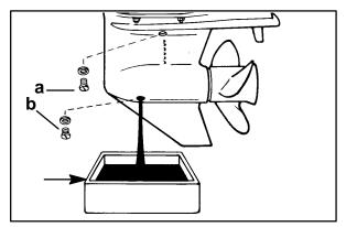
a - Vent Screw w/Sealing Washer
