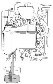
3. Remove 3 bolts securing vapor separator assembly to manifold.
