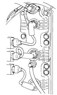
Plug Wire Routing - Starboard Side
