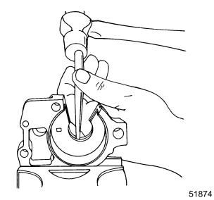
b. Drill two 3/16" (4.8mm) diameter holes thru the top of water pump cover (but not thru insert) at locations shown. Drive insert out of cover with a punch and hammer.
