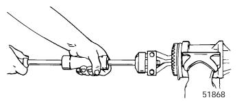
c. If reverse gear bearing remains attached to reverse gear, install Universal Puller Plate (91-37241) and position puller plate, gear and bearing on a press with gear side down. Use a suitable mandrel and press gear out of bearing.
