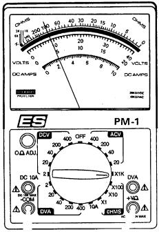
**NOTE:** There are 3 different Multi-Meter DVA Testers using the part number 91-99750 or 91-99750A1 having a DVA built in. Any one of these testers will work with the 135-200 V-6 ignition system.
