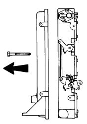
STEP 2: Reattach manifold body without cover to engine using twelve 1/4-20 x 2-3/4" screws in place of screws normally used.
