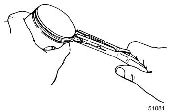
17. Using an awl, scribe identification number of connecting rod on inside of piston (1). Reassemble pis- ton on same connecting rod.
