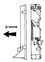
Reattach manifold body without cover to engine using twelve 1/4-20 x 2-3/4" screws in place of screws normally used.
