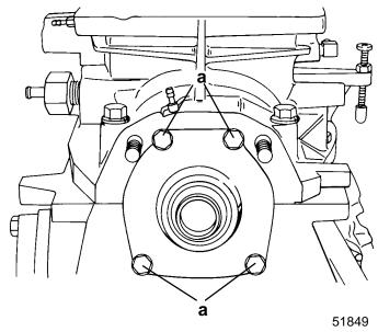
a - Crankcase Attaching End Cap Bolts
