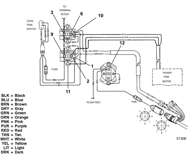
Side Mount Remote Control Wiring Diagram (Test Points for Electrical Troubleshooting)
