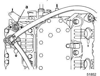
a - Thermostat (143 $^{\circ}$  F 16.7 $^{\circ}$  C)
