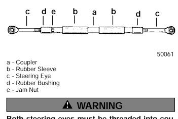
Both steering eyes must be threaded into coupler 3/4 in. (19mm) minimum. Thread length of steering eye is 3-1/2 in. (89mm), so exposed thread must not extend out of coupler more than 2-3/4 in. (70mm). Failure to adhere to this requirement could result in steering system failure.
