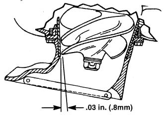
After setting the impeller height, tighten the impeller nut snug with a wrench. Secure impeller nut by bending tabs (a) against the flats on the impeller nut.
