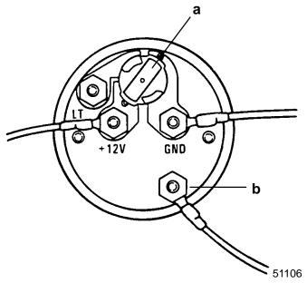
a - Position Light Bulb to the Switched Position b - Sender
