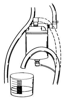
Low or no fuel flow from water separating inlet hose. Perform pulse fuel pump delivery test.
