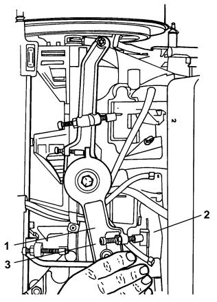
Check preload on throttle cable by placing a thin piece of paper between idle stop screw (3) and idle stop (2). Preload is correct when paper can be removed without tearing, but has some drag on it (readjust throttle barrel, if necessary).
