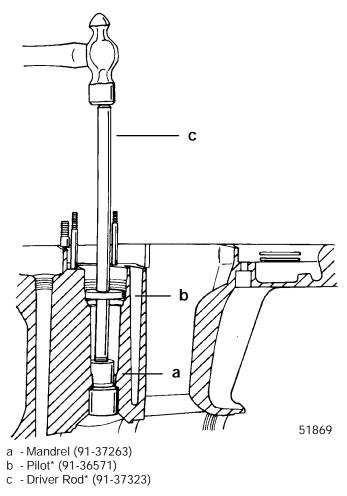
\*From Bearing Removal and Installation Kit (91-31229A5)
