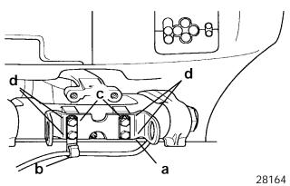
a - Mounting Bracket for Steering Cable Mounting Tube
