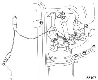
6. Look for leak points on induction manifold while depressing remote starter switch.
