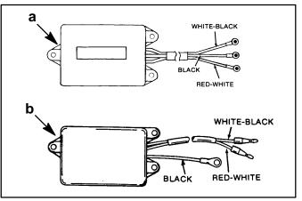
a - Spark Advance Module b - Idle Stabilizer Module
