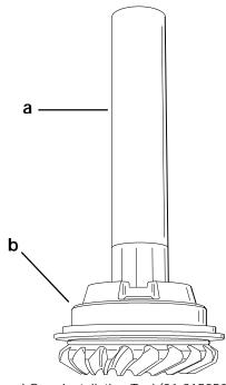
a - Forward Gear Installation Tool (91-815850)b - Forward Gear/Bearing Adaptor Assembly
