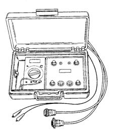
Fuel Pressure Gauge 91-16850 (a) or Fuel Pressure
