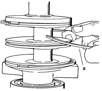
a - Crankshaft Sealing Rings
