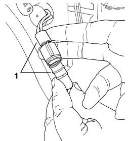
Connect digital using TPS Test Lead Assembly (1) (P/N 91-816085) between TPS connector (2) and EFI harness connector (3). Set voltmeter to 2 DC volts.
