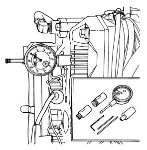
4. Reposition timing pointer (1) (if necessary) so that timing pointer is aligned with .462 in. mark (2) on timing decal. Retighten pointer attaching screws (3).
