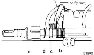
Thread cap (e) onto steering cable mounting tube, up to mark (a).
