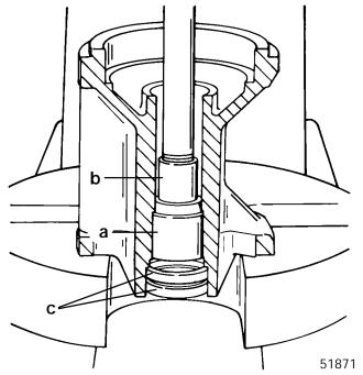
a - Propeller Shaft Needle Bearing
