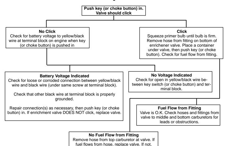
check hose and fitting for leaks or obstructions.
