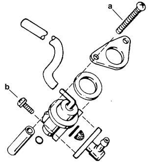
a - Screw (2) [Torque to 30 lb. in. (3.5 N·m)] b - Screw (2) [Torque to 45 lb. in. (5.0 N·m)]
