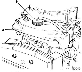
a - Engine Oil Tank b - Fill Cap
