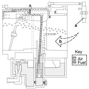
a - Thermal Air Valve (closed)
