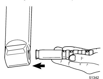
7. Tap shaft into cylinder until shaft is positioned as shown.
