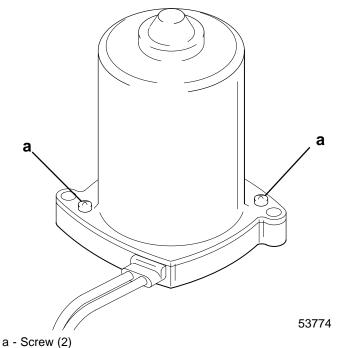
2. Remove frame and armature from end cap. Use
