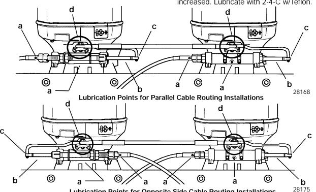
Lubrication Points for Opposite Side Cable Routing Installations
