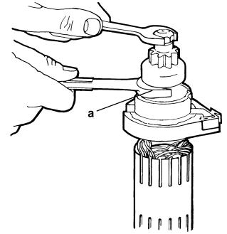
a - Hold Armature Shaft with Wrench on Hex Portion of Drive Assembly Then remove parts from shaft.
