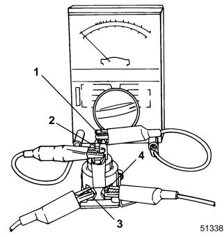
4. If meter does not read zero (0) ohms, replace solenoid.
