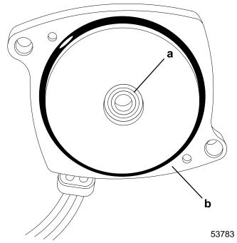
a - Seal (Apply 2-4-C w/Teflon to seal lips)
