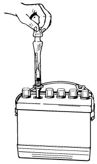
5. Avoid dropping electrolyte on boat or clothing, as it is extremely corrosive. Wash off immediately with baking soda solution.
