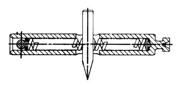
Clutch Actuator Rod with One Additional Shim Washer Added to Each End
