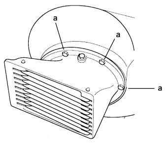
a - Bolts [Torque bolts to 100 lb. in. (11.0 N·m)]
