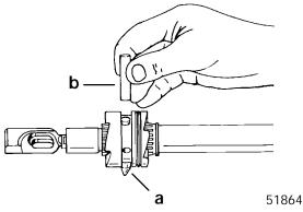
a - Cross Pin Tool (91-86642) b - Cross Pin **NOTE:** Pro Max and Super Magnum models use a slotted cross pin 91-86642-1 and Cross Pin Handle 91-86642-2 to assemble clutch onto propshaft. Turn handle COUNTERCLOCKWISE to install cross pin.
