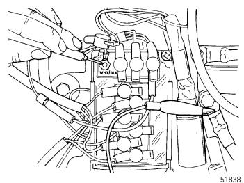
3. Ohmmeter should indicate 1300 - 1500 ohms.
