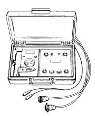
**Results B:** If fuel spray is present using EFI tester, but not present while cranking, perform switch box DVA tests Section 2A (1, 3, 5 switch box failure).
