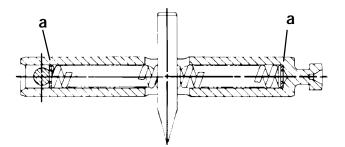
a - Shim only at outer ends of springs as required
