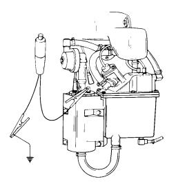
STEP 6: Look for leak points on induction manifold while depressing remote starter switch.
