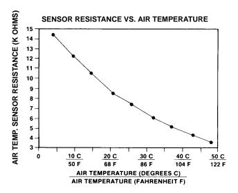
**Results:** Resistance does not change inversely with temperature change. Replace defective Air Temperature Sensor.
