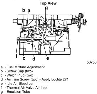
The idle circuit is independent of progression and main circuits. The idle circuit consists of externally adjustable fuel mixture screws, idle air bleed jet, and factory set air trim screws located beneath welch plugs.
