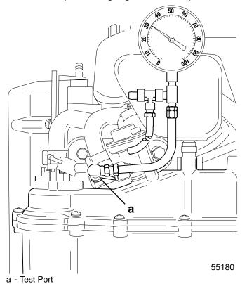
2. Turn ignition key switch to "ON" position and check fuel pressure reading on gauge. If pressure reading is below 34 psi (234 kPa) go to step 3 following.
