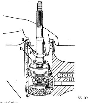
a - Thrust Collarb - Thrust Bearing
