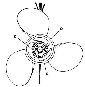
c - Locking Tab Washer (Bend Tabs into Thrust Hub Grooves)
