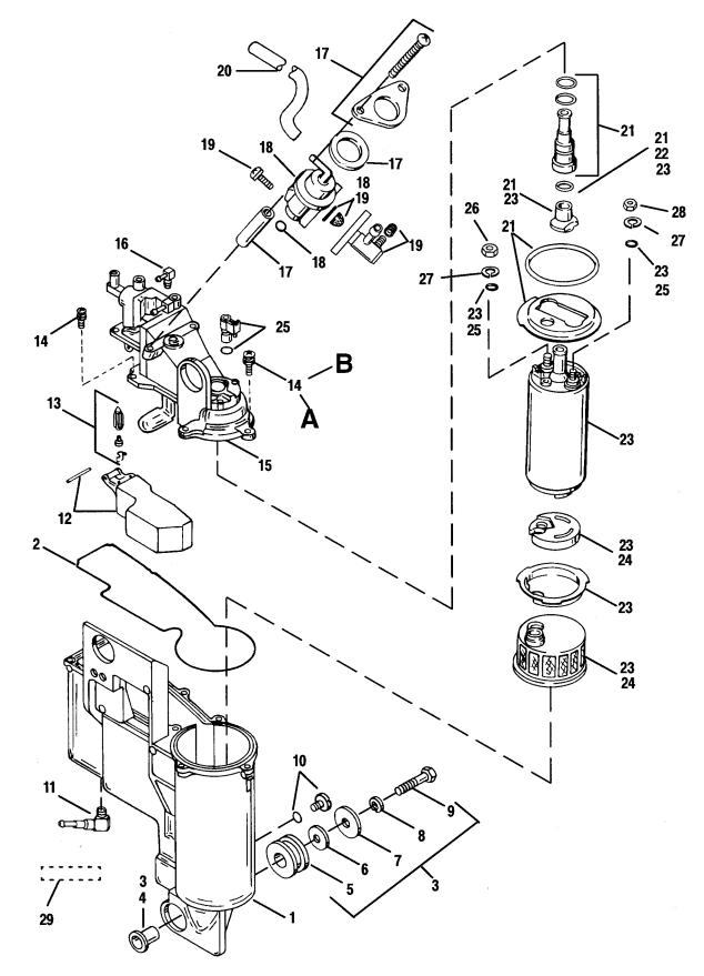
A = LARGE SCREW (5 MM) (TORGUE TO 30 LB. IN. (3.4 N.M) B = SMALL SCREW (4MM)(TORQUE TO 20 LB. IN. (2.3 N.M)
