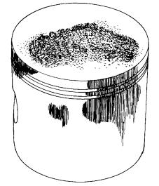
**Damaged Piston Resulting from Detonation**
