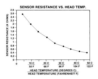
**Results:** Resistance does not change inversely with temperature change. Replace defective Engine Head Temperature Sensor.
