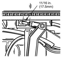
5. Disconnect and isolate white/black lead (a) (starboard side of engine) from 3 wire stabilizer box at bullet connector (b).
