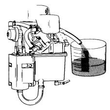
**Results:** If fuel flow is present at hose, remove, disassemble and inspect float assembly. See vapor separator disassembly.
