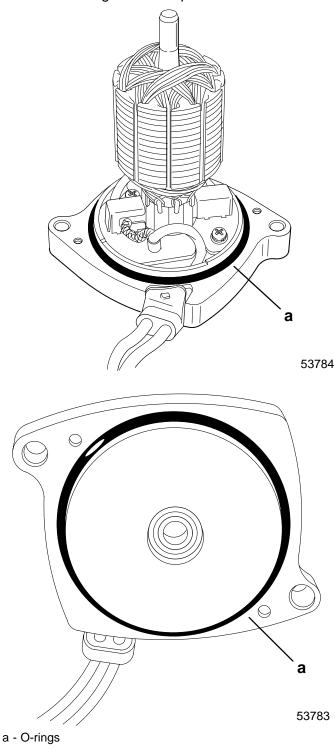
IMPORTANT: Attach Vise Grip® pliers to armature shaft before installing frame assembly. The Vise Grip® pliers will prevent the armature from being drawn out of the brush card assembly by the frame magnets while installing the frame assembly.
