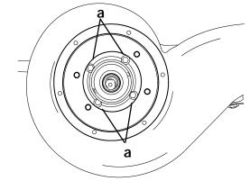
a - Bolts (4) Apply Loctite 271 to Threads, Torque to 70 lb. in. (8.0 N·m)
