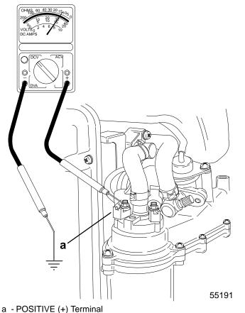
Set volt meter to read battery voltage and connect BLACK test lead to ground, POSITIVE test lead to NEGATIVE (–) post of fuel pump.
