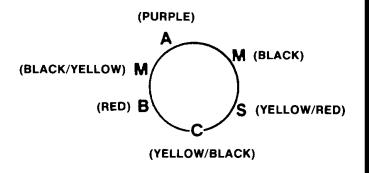
2. Set ohmmeter on R x 1 scale for the following tests:
