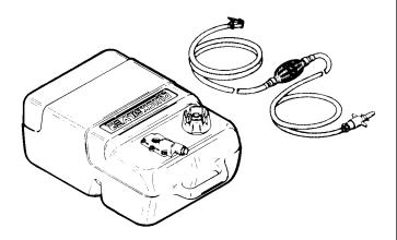
Using a remote fuel tank containing a major brand of premium unleaded gasoline, test run the outboard to eliminate any problems related to restricted fuel supply (clogged lines, malfunctioning anti-siphon valve, etc.) and/or marginal gasoline.
