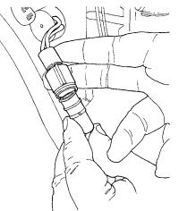
Connect digital using TPS Test Lead Assembly (a) (P/N 91-816085) between TPS connector (b) and EFI harness connector (c). Set voltmeter to 2 DC volts.
