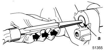
a - Lower Swivel Pin (Remove as shown)
