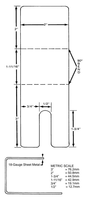
Lubricate bushing (located in commutator end cap) with one drop of SAE 10W oil. DO NOT over lubricate. 8. Place springs and brushes into brush holder and hold in place with brush retainer tool.
