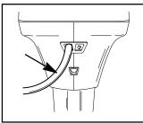
2. Attach a water hose to the fitting. Turn water on and flush for 3 to 5 minutes. DO NOT run the engine when flushing.
