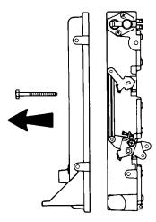
2. Re-attach induction manifold to engine using 1/4-20 x 2-3/4" screws.
