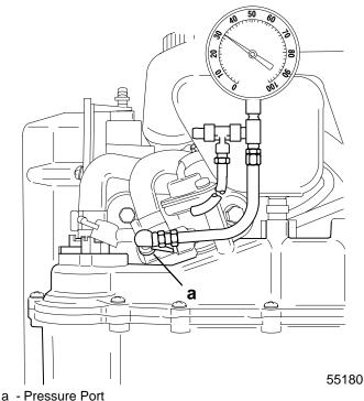
2. Prime engine using fuel primer bulb.
