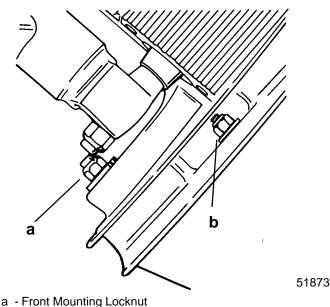
b - Side Mounting Locknut (One Each Side)
