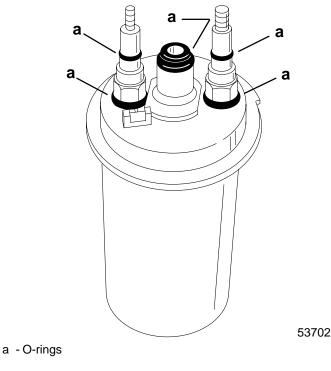
VAPOR SEPARATOR FLOAT REMOVAL
