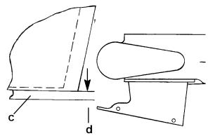
5. Raise the outboard up on the transom the distance measured in Step 4. Use a straight edge and recheck the mounting height. The top edge of the water intake housing should be lined-up with the horizontal line made in Step 1.
