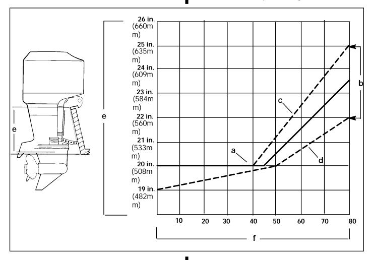
**NOTE:** Add 5 in. (127mm) for XL models and 10 in. (254mm) for XXL models to listed outboard mounting height.
