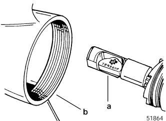
a - Shift Cam (Position as Shown)b - Gear Housing
